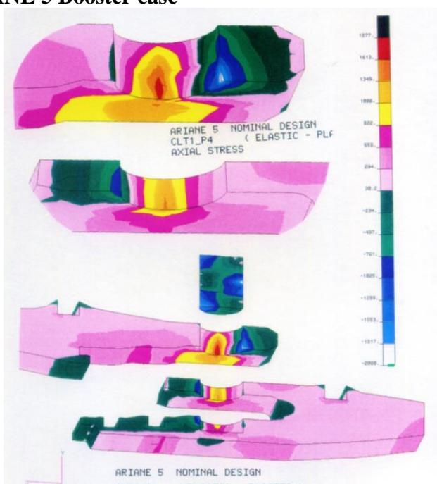
Optimization of the booster case structure of the ARIANE 5 rocket engine and the justification of design criteria based on fracture mechanics
