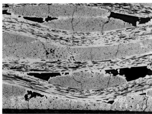
Investigations of the failure behaviour of fibre strengthened ceramic materials (CMC: Ceramic Matrix Composite)
