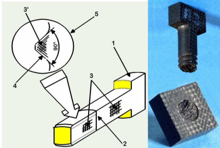
Structural materials, manufacture and design of metallic (refractory) and ceramic high temperature bolt elements for the application in the space structures, particularly for the light weight CMC structures
